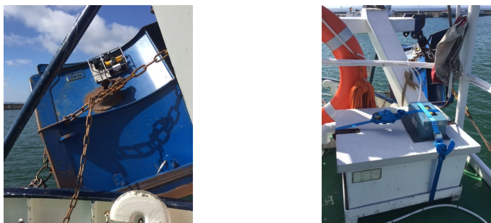
Figure 2 mountings: data logger at trawl door (left) and GPS logger on deck (right)
